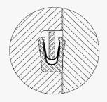
As the seal also will have pressure from behind, the choice was to use two V-shaped springs in the spring groove.
