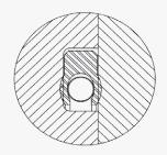
To seal efficiently against gas, a powerful helical spring is applied.
